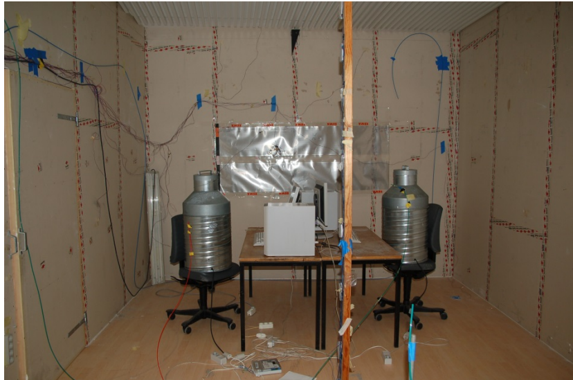
The test room for measurement of ventilation efficiency and indoor thermal comfort in building 119
